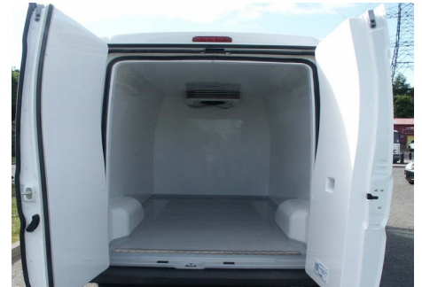
Interior showing evaporator installation plus interior panels
