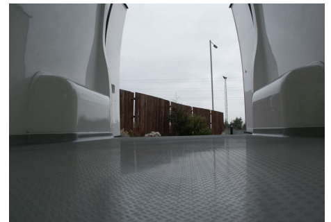
One-piece floor showing edging providing sealed floor unit and one-piece panel high gloss finish construction
