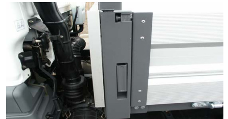
Over centre swinging side board fasteners
