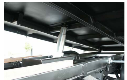
Multi-stage ram, fully welded sub frame
